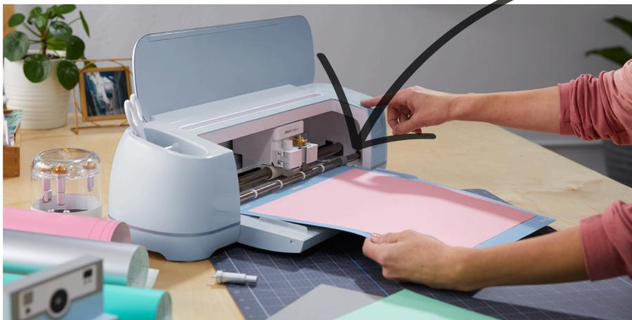
Don't forget to put the mat under the mat guides!
